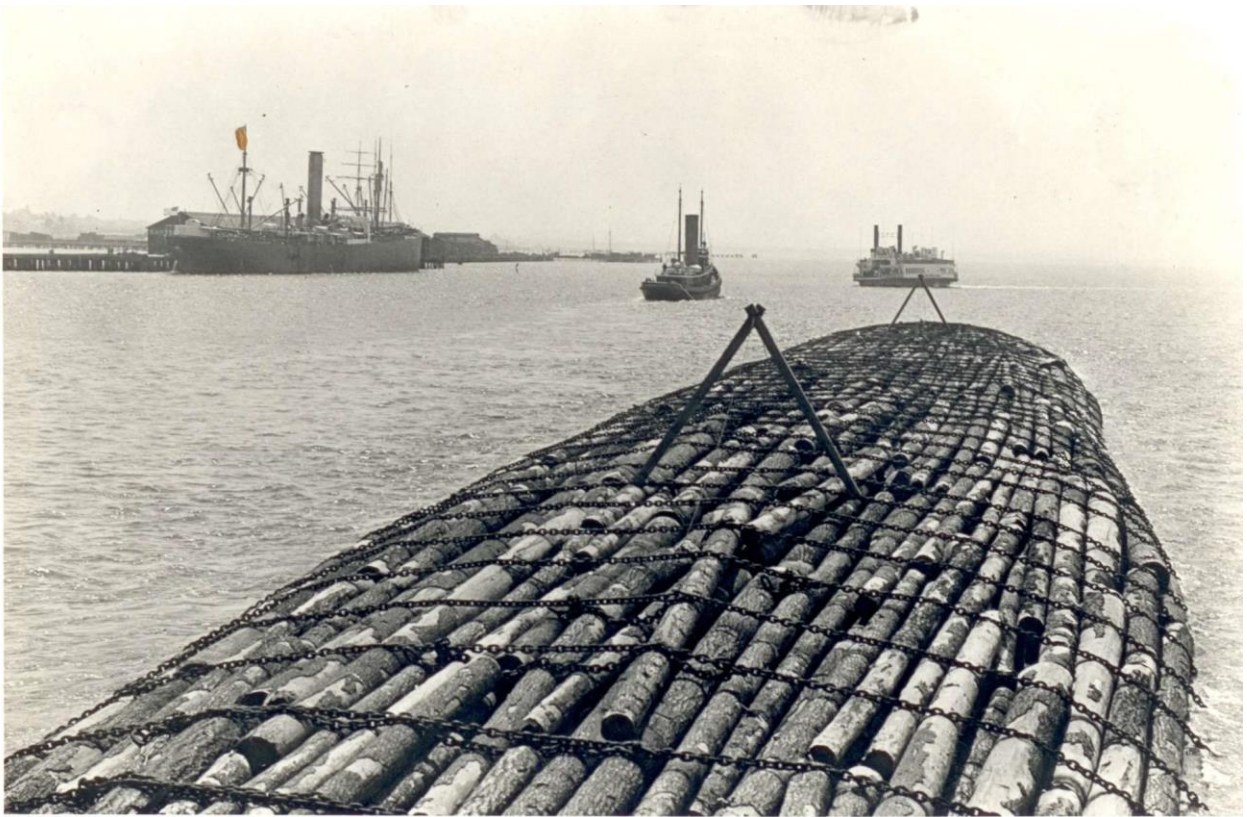
A 900-foot log raft, under tow by the tugboat Hercules (center), on the way to the Benson saw mill in San Diego Bay, circa 1910. Courtesy Maritime Museum of San Diego.
